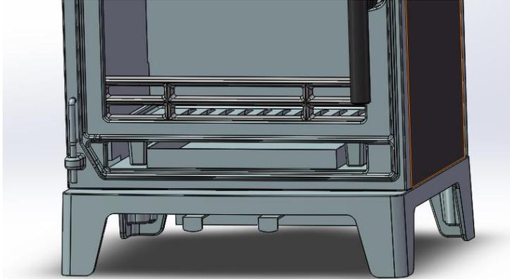
3. Adjust the stove leveling bolts show picture below until the stove is level and evenly supported. Take care not to damage the floor surface.
