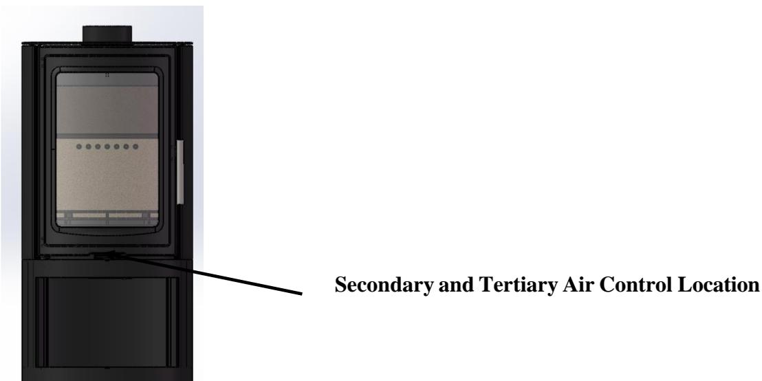
The control has an internal rotary plate with slots, housed inside the body of the appliance and is located below the right-hand corner of the fire door assembly, when looking at the front of the appliance.
