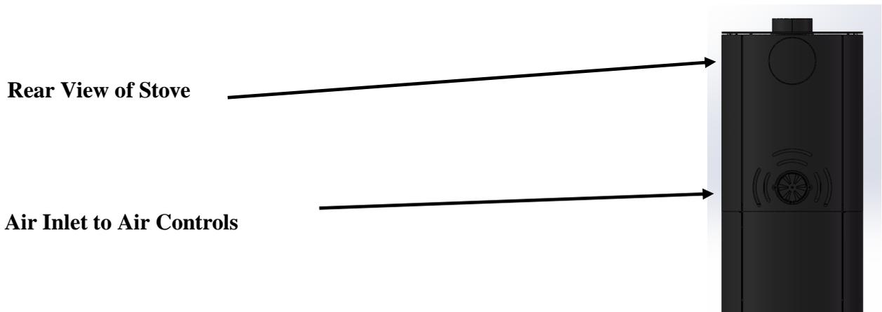
NOTE: DO NOT COVER OR PARTIALLY OBSTRUCT THE AIR INLET OPENINGS FOR THE APPLIANCE
